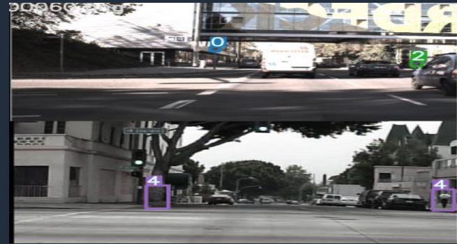
Fig 6. Pedestrian and sign detections by trained detector.
