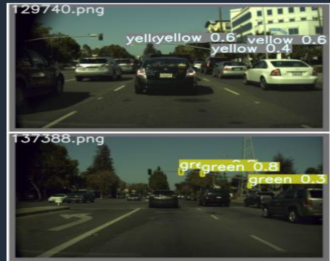
Fig 5. Traffic light detections by trained detector.
